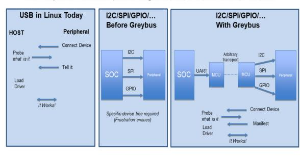
$BeagleConnect^{\mathsf{TM}} \ uses \ Greybus \ and \ mikroBUS \ add-on \ boards \ with \ ClickID \ and \ BeagleConnect^{\mathsf{TM}} \ mikroBUS \ manifests \ to \ eliminate \ the \ need \ to \ add \ and \ manually \ configure \ devices \ added \ onto \ the \ Linux \ system.$
